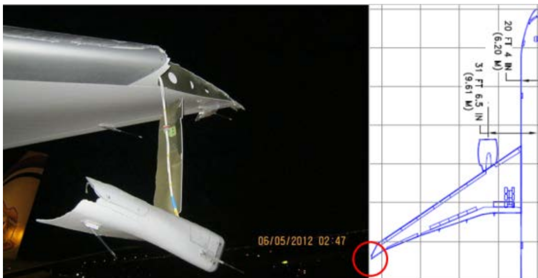
Figure 3 B777 LH Wingtip Damage
