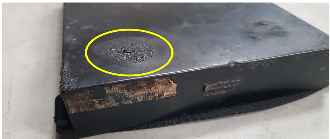
Figure 3: Burn marks on battery body, in relation to visible burn marks on housing
