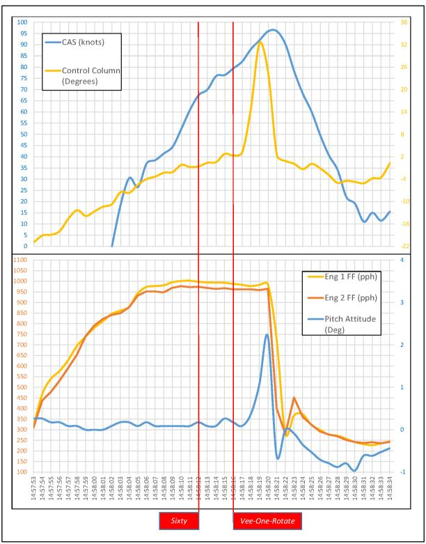
Note. The elevator position attained was sufficient to rotate an aircraft loaded within the operational CG envelope (elevator position not presented in this plot).
