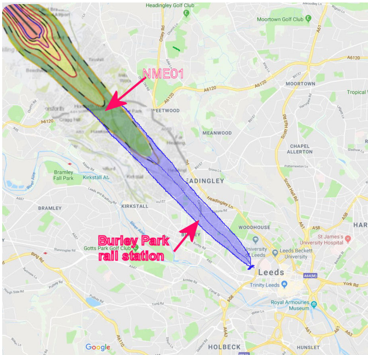
Figure 2: Our Best estimate of impact of Shallower Ascent Profiles on Aircraft Noise at Ground Level (54 Db L_{Aeq} 16hr)
