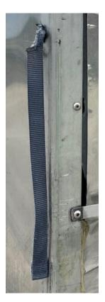
The probability of a serious fall should one of these straps fail during use, is extremely high. Over the years, there have been more than one fatal accident involving ground staff falling backwards off high loaders, when a pull strap fails suddenly during use.
